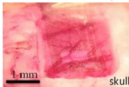
Fig. 1. Organic transistor array recording epileptic seizures from the cortex of a rat
